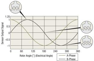
Output Signal of Rotor Position Detection Sensor
