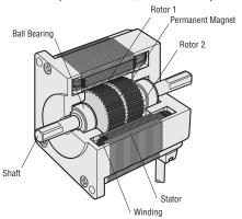
Motor Structural Diagram: Cross-Section Parallel to Shaft
