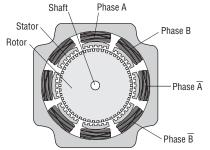
1.8° Stepper Motor Structural Diagram: Cross-Section Perpendicular to Shaft
