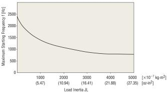
Inertial Load - Starting Frequency Characteristics
