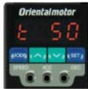
The Display when the Load Factor is 50%
