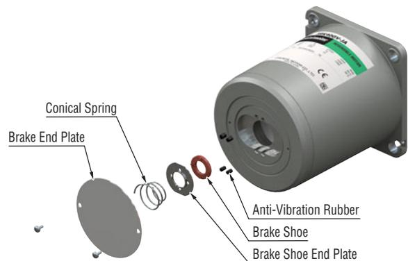
From a structural perspective, applying a constant load to the brake shoe allows it to slide. The structure of the brake shoe is integrated to reduce deterioration with age, and the materials used are resistant to wear.
