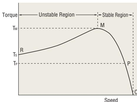
Under no load, the motor rotates at a speed close to synchronous speed. As the load increases, the motor's speed drops to a level (P) where a balance is achieved between load and motor torque ( $T_r$ ). If the load is further increased and reaches point M, the motor can generate no greater torque and stops at point R. In other words, the motor can be operated in a stable range between M and O, while the range between R and M is subject to instability.
