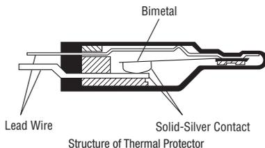
The thermal protector employs a bimetal system in which solid silver is used in the contacts. Solid silver has the lowest electrical resistance of all metals and has the second highest heat conduction second only to copper.
