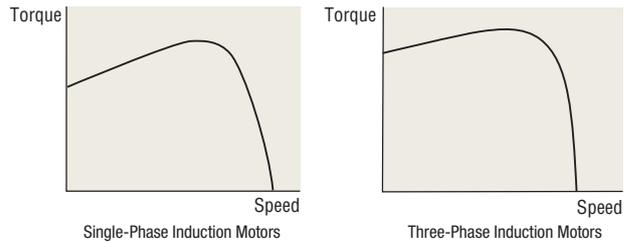
The torque the motor produces changes proportionally to roughly twice the power supply voltage. For example, if 110 VAC is applied to a motor whose rated voltage is 100 VAC, the torque produced by the motor increases to approximately 120%. In this case, the motor temperature will rise and may exceed the permissible range.
