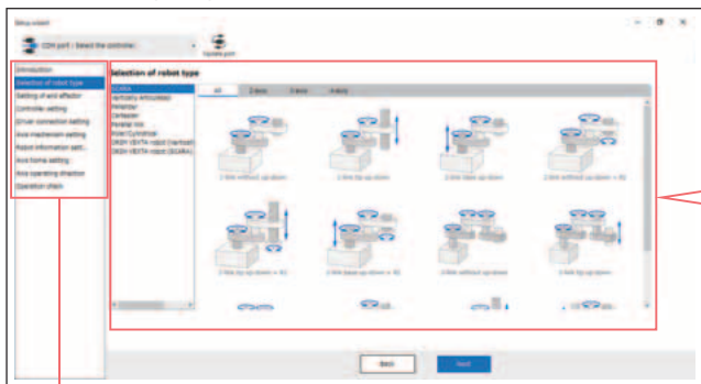
Proceed through initial setting of the robot by following the wizard menu.
