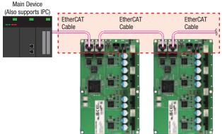
The right-angle connector direction type can be installed with several units placed side by side, eliminating crowded wiring and saving space.
