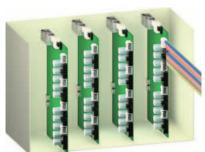
Driver connector positions are concentrated on two sides. This simplifies wire bundling.
